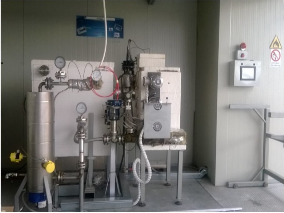
Fig. 2. The PROGEO apparatus: a methanation prototype reactor working in the Laboratory of Chemical Technologies of the DICA – University of Perugia (Italy).
